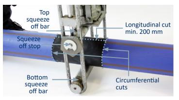
Fig 3. Position of the longitudinal cut, relative to the squeeze off bars
