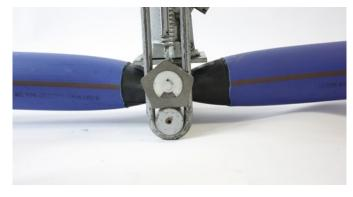
Fig 6. Pipe in the fully squeezed position.
