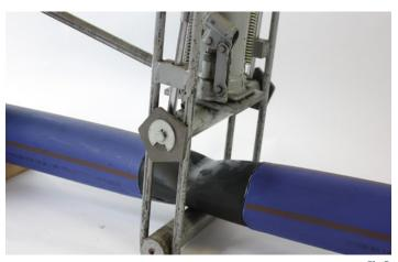
Fig 8. Tool fully open ready for removal
